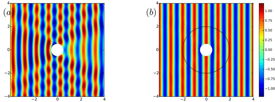
Figure 2: Scattered field of waves in the presence of a cylinder without a cloak (a), and with the cloak (b). The black circle in figure (b) shows the boundary of the cloak.
