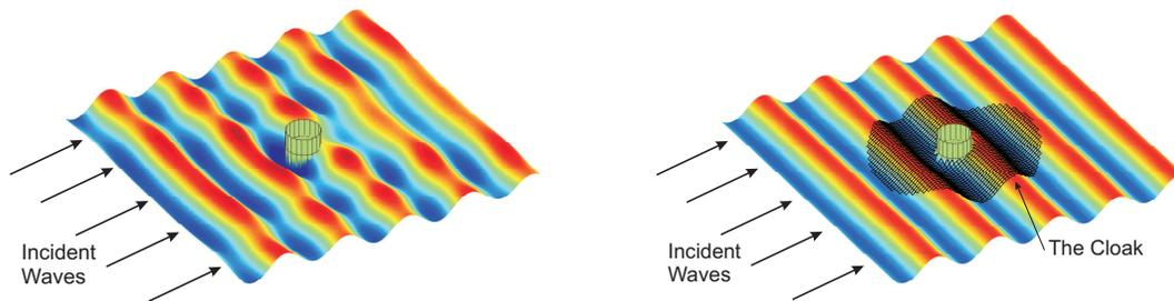
Figure 1: Figure (a) shows the scattering pattern of a cylinder under the action of water waves without a cloak, and figure b. shows the same cylinder protected by a surface wave cloak. Clearly in figure (b) there is no scattering and the cylinder is *cloaked*.
