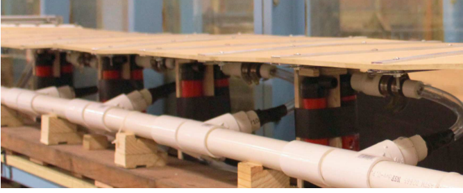
(a) The white PVC pipe connects all ten pumps (red cylinder) with the PTO discharge where the generated flux is measured. Two pumps are creating one double reacting PTO unit.
