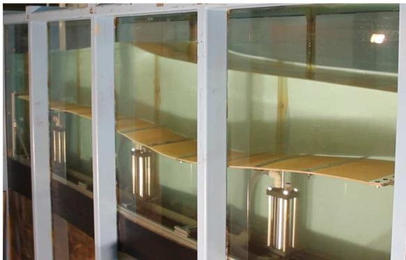
**Figure 4:** A photograph of the wave tank and the wave carpet along with the PTO.
